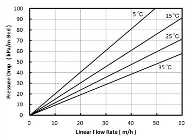
Fig. 2 Pressure Drop of SP850
