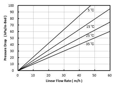
Fig. 2 Pressure Drop of HP21
